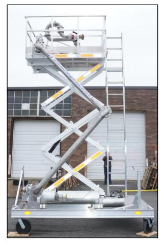
High Reach Scissor Lift Pantograph is an Aviation Refueling Equipment for military and commercial aircraft. It is mainly designed to support underwing refueling of wide body aircraft. The towable and movable stainless-steel scissor lift platform with the dispensing end is easily extended up to a connection height of 19 ½ feet maximum above ground level.
